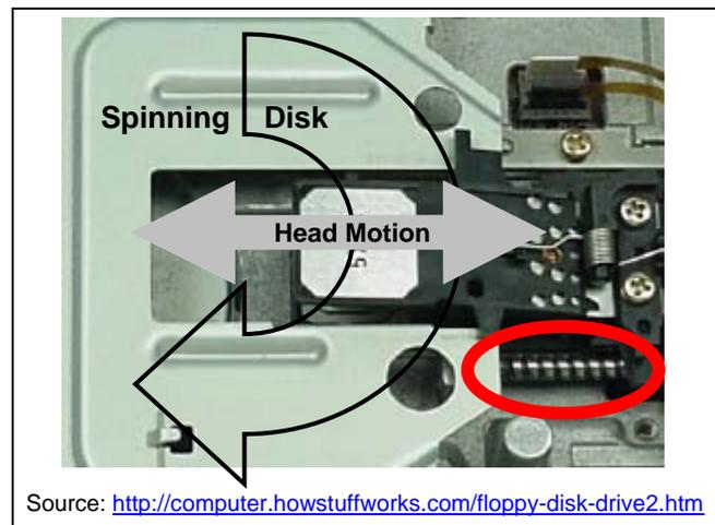
**Illustration 1:** As the disk spins, the screw (circled) moves the head back and forth over the spinning disk.
